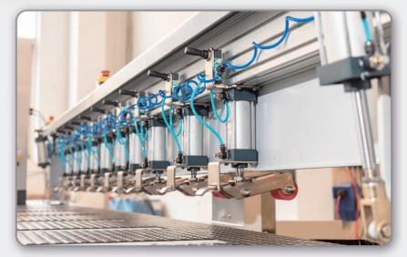
10 pneumatic fixtures to hold the stone in position are included in the machine, they can be moved manually according to the position of the stone, and they are locked and released easily
