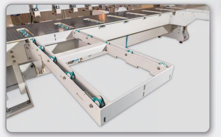
This holder supports longer stone pieces preventing them to brake or crack. The size of the supplementary holderis 600mm x 1100mm.
