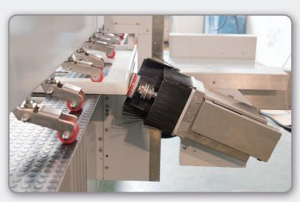
The machine is supplied with a toolpresetting system that can measurethe thickness of the grinding toolautomatically.
